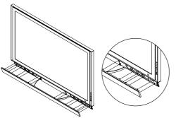
Connect the speakers to the PDP using the speaker cable.The connection terminals are on the rear side of both the PDP and the speakers. (Match the color coded terminals and cables.)
